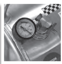
Built-in pressure gauge shows tank pressure
